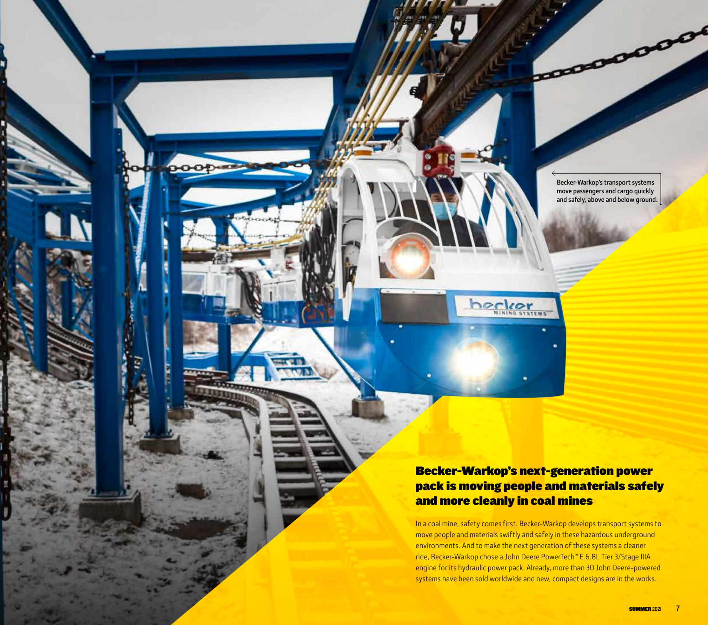
Becker-Warkop's transport systems move passengers and cargo quickly and safely, above and below ground.
