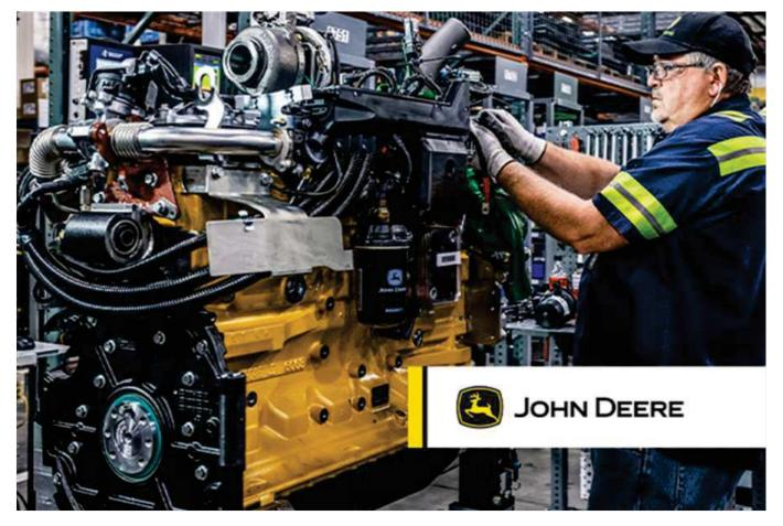
In the off-highway industry, where power and reliability are paramount, equipment owners are increasingly turning to remanufactured parts to avoid downtime. Remanufacturing is a comprehensive industrial process that returns a worn-down or failed part to like-new quality. Manufacturers like John Deere leverage remanufactured parts as a cost-effective repair solution over the lifetime of a piece of equipment. Reman parts, often overlooked in favor of brand-new components, offer a host of benefits.
